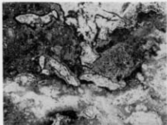
Fig. 8. The polycrystalline quartz mosaics in this specimen (light areas) appear to be relics of large quartz crystals from the original granite. Feldspar is completely reconstituted into fine fibrous aggregates and occasionally into nests of more distinct crystals. The dark material seems to be hematite-stained glass. Plane polarized light. Long dimension of field is 6.1 mm.
