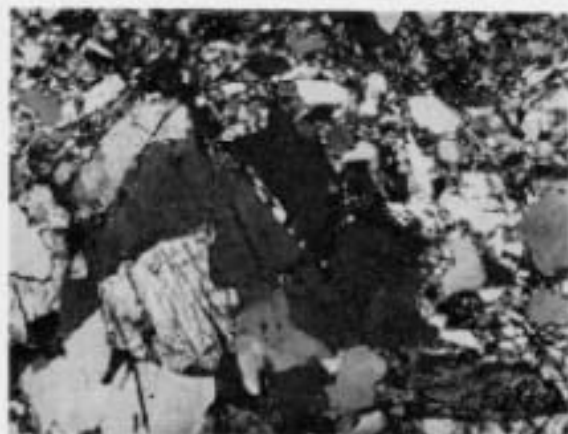
Fig. 1. Margin of a clast of hornblende quartz-diorite in microbreccia. Hornblende grain near bottom right. A large quartz crystal is seen in the process of breaking into angular fragments. The fractures, which have opened and filled with shards of quartz and feldspar, are in this case approximately parallel to the c -axis. Crossed polarizers. Long dimension of field is 6.3 mm.
