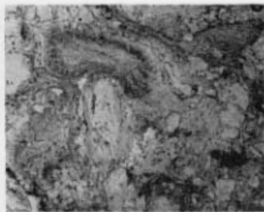
Fig. 7. In hand specimen, this rock appears to be a slightly decomposed granite, but it is completely reconstituted. The ovoid cloudy areas shown here are quartz, which under crossed polarizers is seen to be recrystallized into a polycrystalline mosaic. The feldspars are partly aggregates of fine fibers and sheaf-like bundles, and partly recrystallized into decussate masses of distinct individuals. The patterns of distortion within the original feldspar crystals are clearly visible where the new microclites are small, but are lost when the new crystals grow larger. The feldspars evidently flowed around and between the quartz areas, which seem to have preserved their unity. This field, under crossed polarizers, is illustrated in N. M. Short (1966, Fig. 11); the magnification given there should be 18X). Plane polarized light. Long dimension of the field is 4.9 mm.
